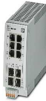
4/12 puertos RJ45, 2 puertos SFP y 2 puertos Combo Fast Ethernet 10/100 MBit/s
