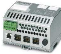
1 puerto RJ45 y 3 puertos POF SC-RJ
